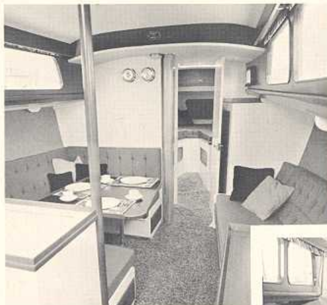
(Above, right) Tomboy's cockpit... (above) main cabin, looking toward forward stateroom. Settee makes into a double berth... (right) main cabin looking aft. Galley has two-burner range with oven, ice box, chart table over quarter berth
